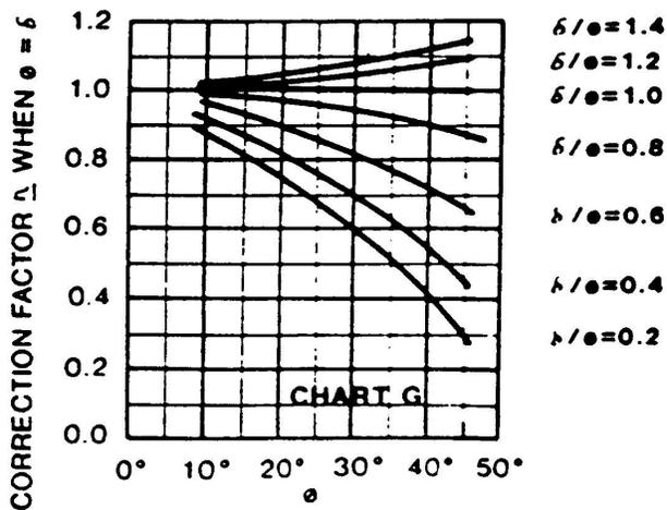
Figure 9. Friction factors for piles in granular soil; friction angle  $\delta$  for sand on steel = 18.5° (for piles with no appreciable taper).
